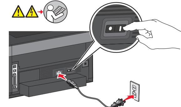
Connect the power cable to the printer and then to the wall. Turn on the printer.
